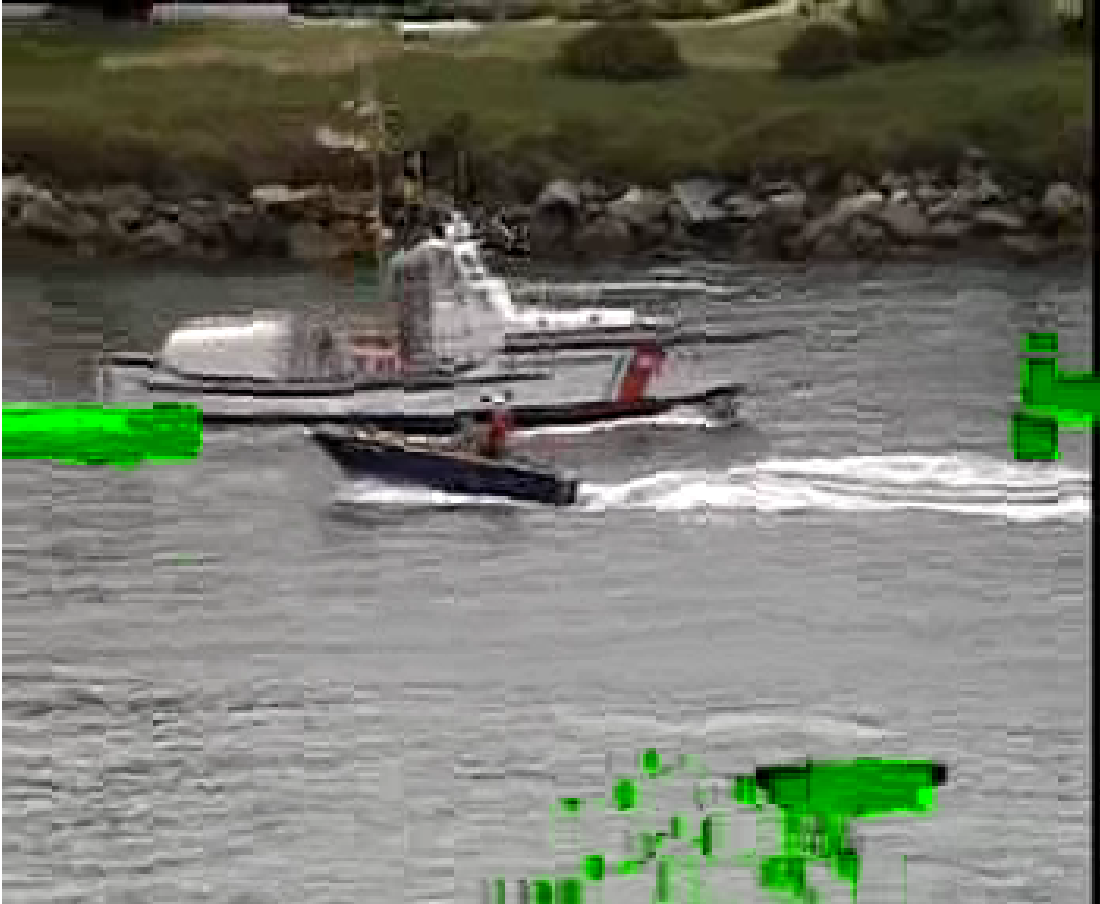
Figure 3-2: B-frame #65 from “coastguard” stream showing propagation of errors. Y PSNR = 17.538345
