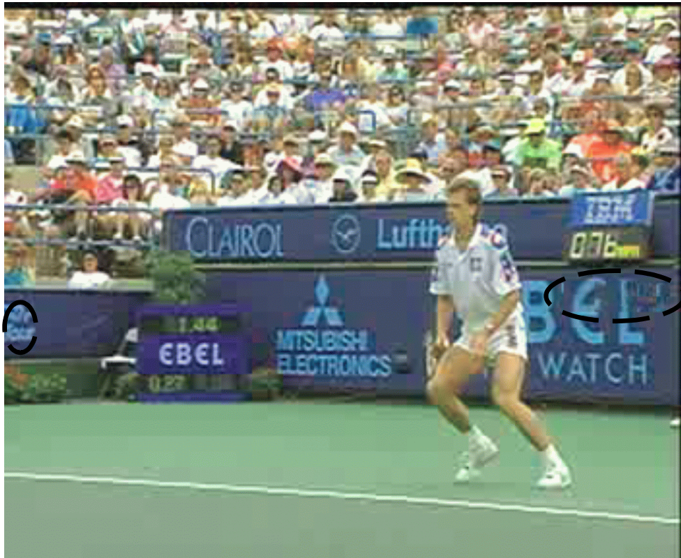
Figure 3-18: I-frame Packet Loss Recovery making use of motion information. Reconstruction of the damaged region is much more accurate.
