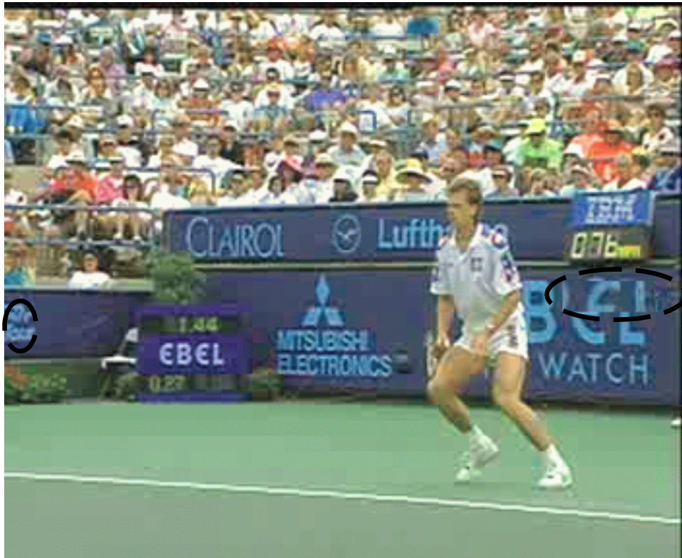
Figure 3-17: I-frame Packet Loss Recovery using Simple Replacement. While this works well for scenes with low motion, distortion is quite noticeable in the area containing the “EL” characters.
