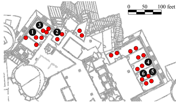
FIGURE 3-7—Experimental Zigbee testbed layout: there are 31 nodes in total, spread over 11 rooms in an indoor office environment. Each unnumbered dot indicates one of 25 Zigbee nodes. The six software defined radio nodes are shown dark, labeled with numbers.
