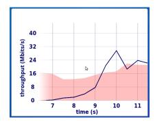
Figure 2: LinkShell supports live graphing of network usage, comparing the link capacity of the input traces (red shading) to the amount of data a client application attempts to transmit (blue line).
